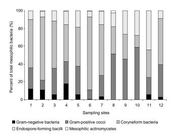
Figure 1. Composition of mesophilic bacteria isolated from the air of a sewage treatment plant (total count).
